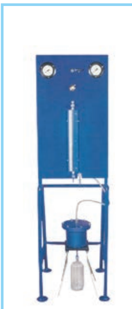
CONCRETE PERMEABILITY APPARATUS
