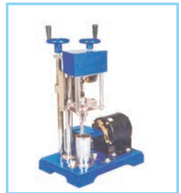
LABORATORY VANE SHEAR APPARATUS (LABORATORY PURPOSE.)
