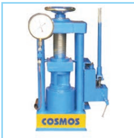
Compression Testing Machine (Manual)
