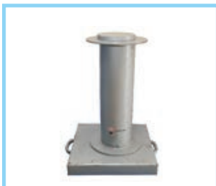
SAND REPLACEMENT EQUIPMENT (SAND POURING METHOD)
