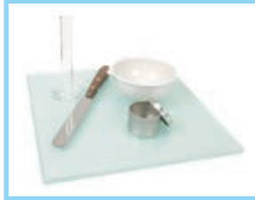
SHRINKAGE LIMIT TEST APPARATUS
