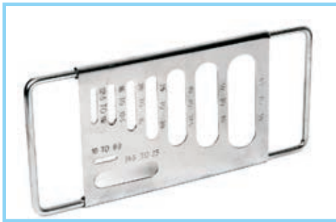
THICKNESS GAUGE / FLAKINESS GAUGE
