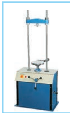
LABORATORY C.B.R. APPARATUS (HAND OPERATED.)
