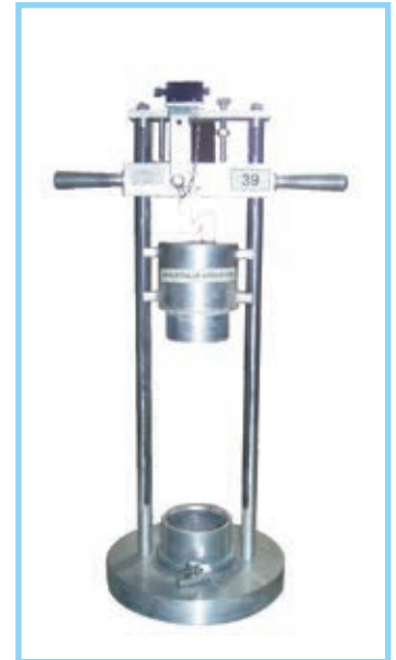
AGGREGATE IMPACT TESTER
